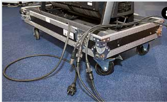
08 / Dedicated connectors are waterproof (IP65), and adapters are included.
