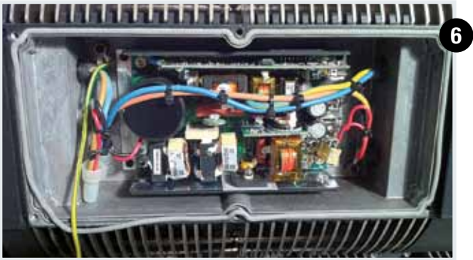
06 / One of the four high-class power supply with active PFC, carefully protected from external aggressions.
